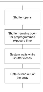
Figure 28. Free Run {No Response} Timing Chart, part of the chart in Figure 36
